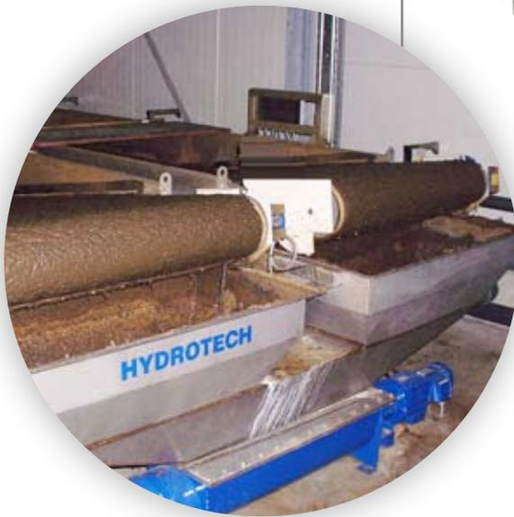
*Two or more Beltfilters can be used in parallel when a higher filtration capacity is required.*
